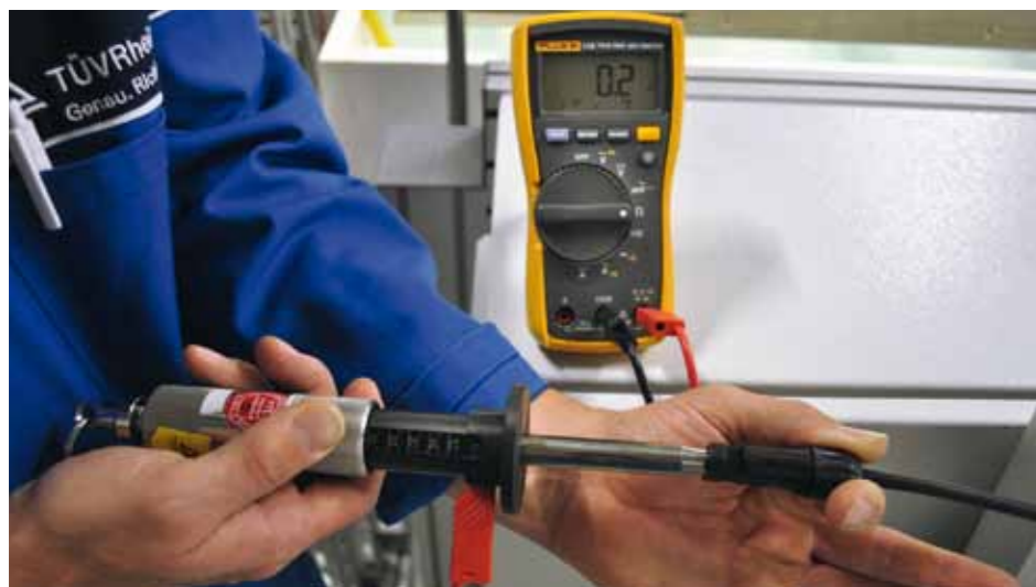
In two of the five test modules from the Chinese manufacturer who chose to remain unnamed, the contacts of the male plug connector were able to be contacted with a test finger. A no-go!
